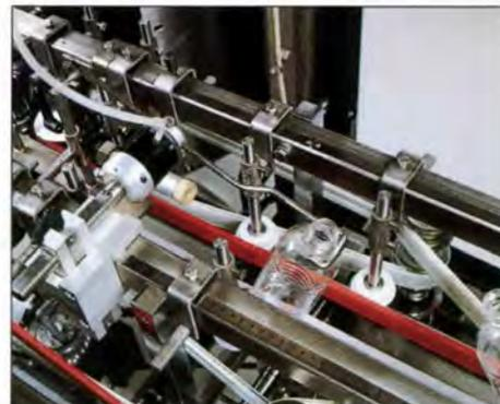
*A linear bottle path enables accurate positioning as bottles approach the qualifying arm.*
